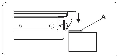
Place the sealing gasket A all around the edge of the cut out.
