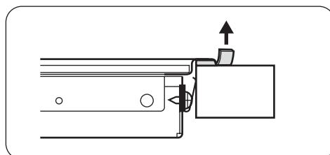
Fit the hob in the cut out and push it down until it comes in contact with the kitchen top surface. then remove the excess sealing.
